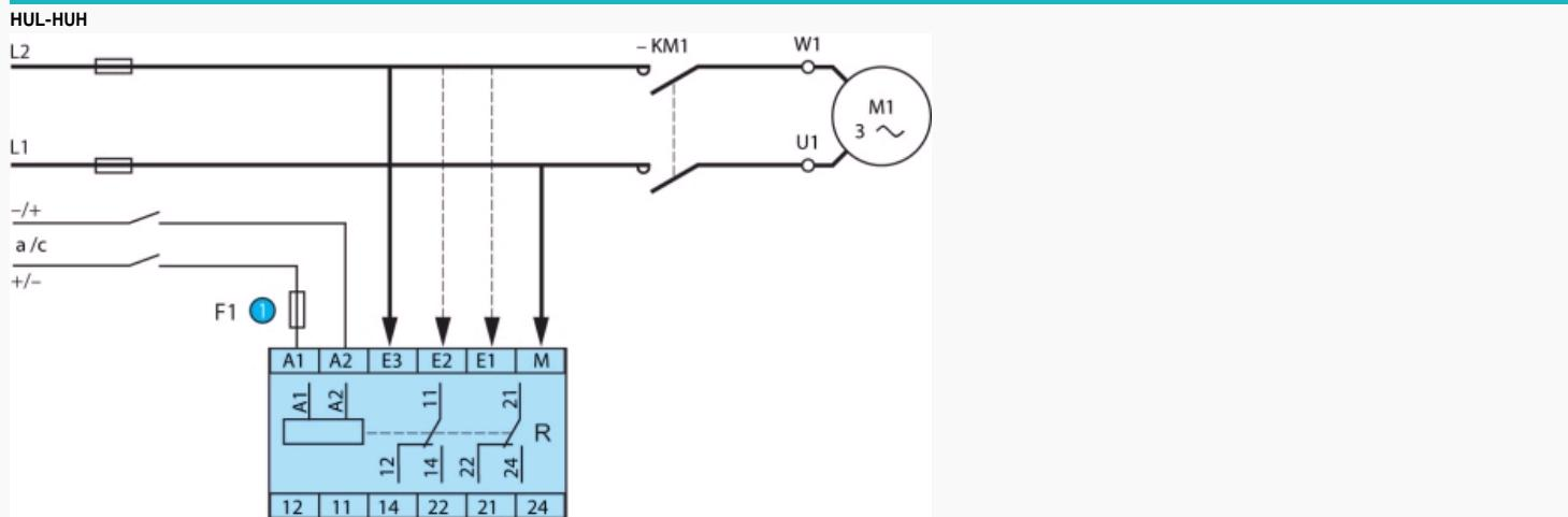
NB : When controlling DC voltage from the same source supplying terminals A1 and A2, terminal M must be connected directly to the "minus" pole of this power supply.
