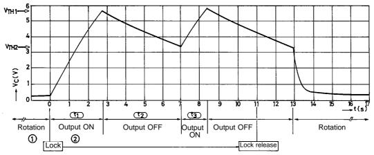
Automatic Return Circuit C Pin Voltage
