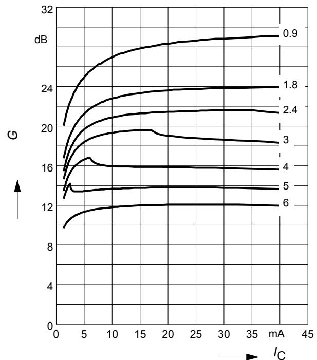
**Power gain  $G_{\text{ma}}, G_{\text{ms}} = f (V_{\text{CE}})$**
