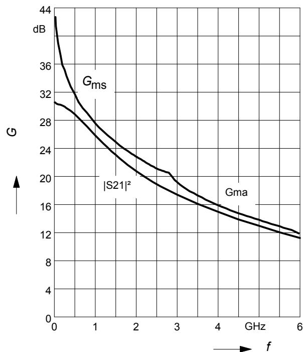
**Power gain  $G_{\text{ma}}, G_{\text{ms}} = f (I_{\text{C}})$**
