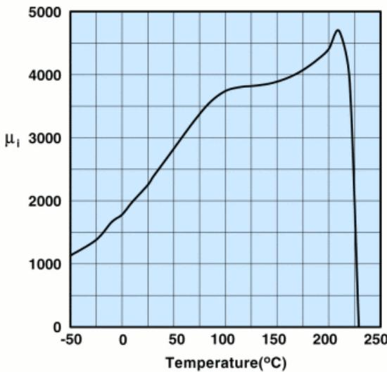
Measured on an 18/10/6mm toroid at 100kHz.
