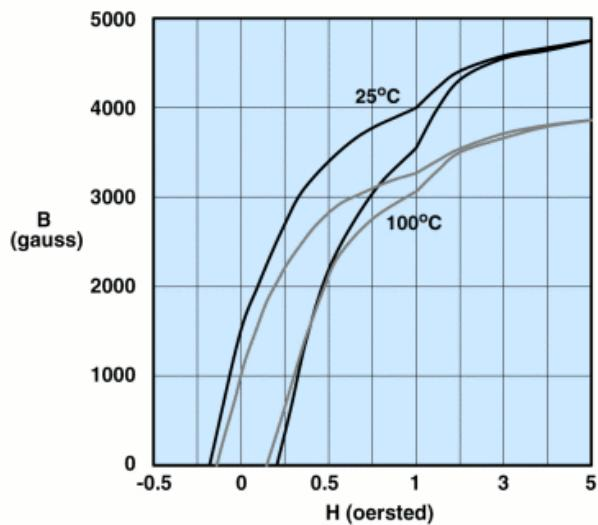
Measured on an 18/10/6mm toroid at 10kHz.
