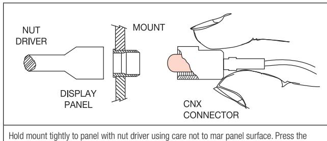
Hold mount tightly to panel with nut driver using care not to mar panel surface. Press the connector with LED into place.
