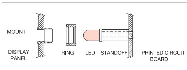
Hold the mount to the panel securely while pressing the retaining ring into position with a nut driver. A standoff may be used for proper LED height adjustment. Slide PCB mounted LED into position.
