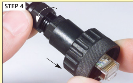
Slide crimped connector into place and tighten compression nut.
