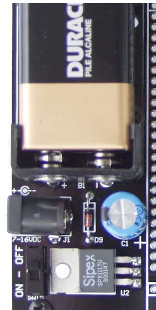
Figure 9: The Decoder Board Power Supply Area
