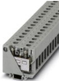
Feed-through terminal block, Connection method: Screw connection, Cross section: 0.5 mm 2 - 10 mm 2 , AWG 20 - 8, Width: 7.5 mm, Color: gray, Mounting type: NS 15
