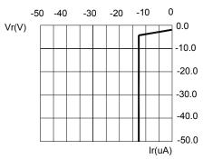
FIG.2 REVERSE CURRENT VS. REVERSE VOLTAGE.
