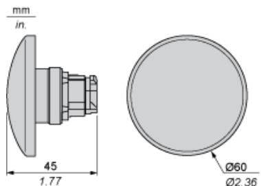
Heads for Double-Headed, Spring Return Pushbuttons
