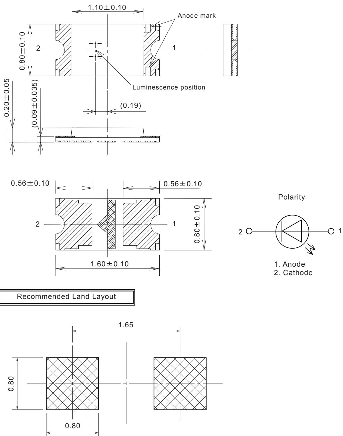
(Note1) Electrode projection is not included in the package dimensions.
