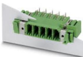
Feed-through header, nominal current: 41 A, rated voltage (III/2): 630 V, nominal cross section: 6 mm<sup>2</sup>, number of positions: 5, pitch: 7.62 mm, color: green, contact surface: Tin, mounting: Wave soldering, pin layout: Linear pinning, solder pin [P]: 4.26 mm
