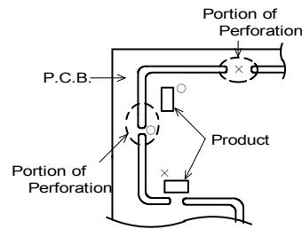
The portion of perforation shall be designed as narrow as possible, and shall be designed so as not to be applied the stress in the case of P.C.B. separation.
