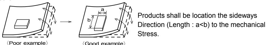
Products shall be located the sideways Direction (Length : a<b) to the mechanical Stress.
