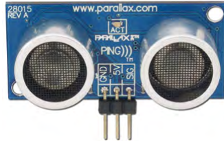
Figure 2-1 The Ping)))™ Ultrasonic Distance Sensor
