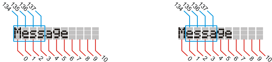
Figure 1-21: Shifting Text Through Window, Steps 3 and 4
