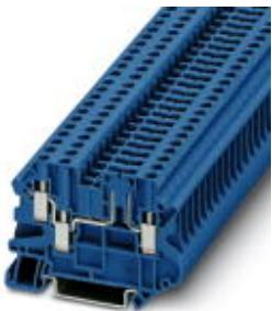
Feed-through terminal block, Connection type: Screw connection, Cross section: 0.14 mm<sup>2</sup> - 6 mm<sup>2</sup>, AWG: 26 - 10, Nominal current: 20 A, Nominal voltage: 500 V, Length: 65.4 mm, Width: 6.2 mm, Color: blue, Assembly: NS 35/7,5, NS 35/15
