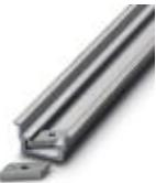
DIN rail, deep drawn, high profile, unperforated, 1.5 mm thick, material: aluminum, height 15 mm, width 35 mm, length 2000 mm
