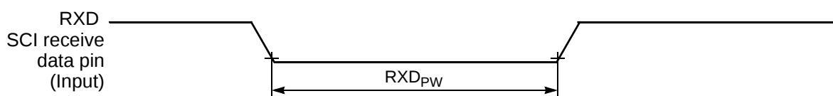
Figure 10-15 RXD Pulse Width
