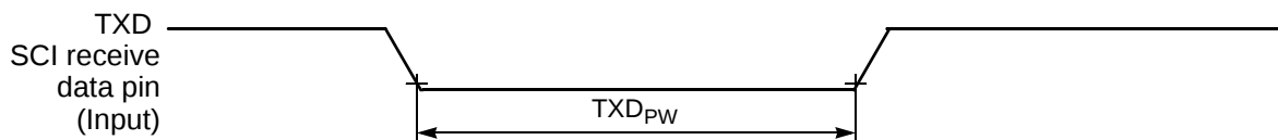
Figure 10-16 TXD Pulse Width
