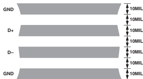
Figure 4. Arrangement of Signal Tracks
