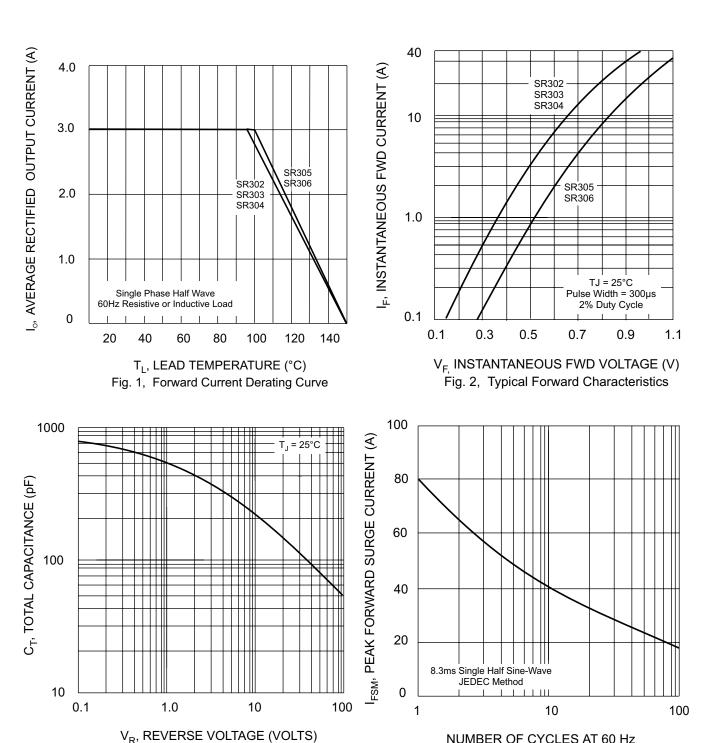
NUMBER OF CYCLES AT 60 Hz Fig. 4, Max Non-Repetitive Peak Fwd Surge Current
