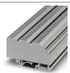
Feed-through terminal block, nom. voltage: 800 V, nominal current: 20 A, connection method: Screw/plug-in connection, number of connections: 4, number of positions: 1, cross section: 0.2 mm² - 4 mm², AWG: 24 - 12, width: 7.62 mm, color: gray, mounting type: NS 35/7,5, NS 35/15, NS 32
