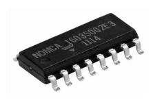
The NOMCA series features a standard 14 pin or 16 pin narrow body (0.150") small outline SMT package. The network is constructed with tantalum nitride resistor film on high purity alumina substrate for improved ESD and moisture protection. Custom schematics are available consult factory.
