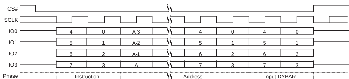
Figure 10.63 DYBWR QPI Mode Command Sequence
