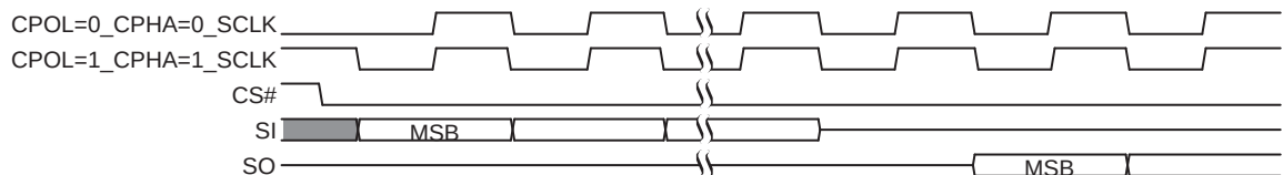
Figure 4.1 SPI SDR Modes Supported
