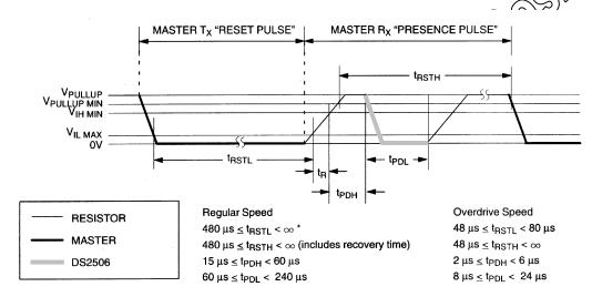
\* In order not to mask interrupt signalling by other devices on the 1-Wire bus,  $t_{RSTL} + t_R$  should always be less than 960  $\mu$ s.
