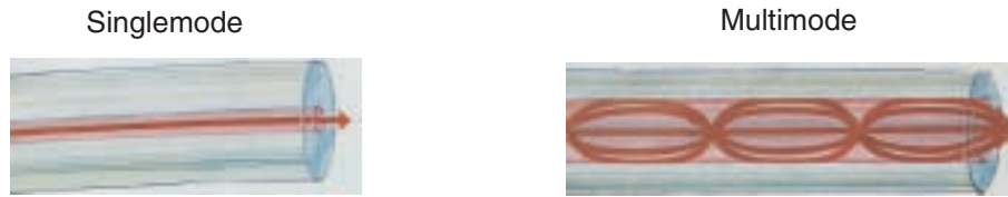
Figure 2. Singlemode and Multimode Fibers
