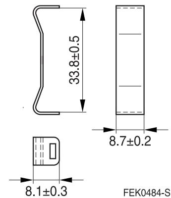
**Coil former (magnetic axis vertical)**
