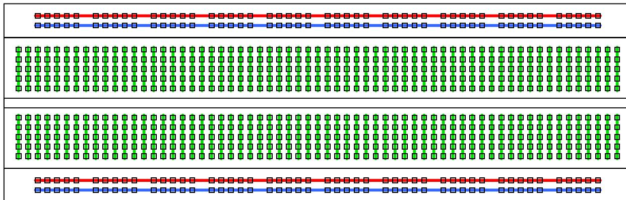
The BB830 and BB830T breadboards have 63 vertical columns on top and 63 columns below. Each column has 5 connected holes each (the green lines). This is the circuit area. There are also 4 "rails" (or distribution strips) for power and ground running horizontally (the red and blue lines).
