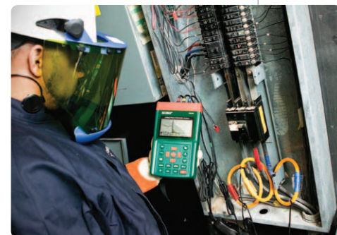
PQ3350 3-Phase Power & Harmonics Analyzer
