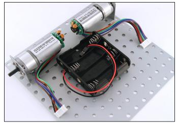
4. Attach the Pmod clips to the metal platform on either side of the battery holder.
