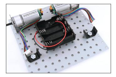
5. Attach the drag button to the metal platform, below the battery holder.
