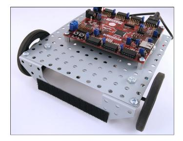
14. Cut four ½-inch sections of Velcro from the other 4-inch strip. Attach these ½-inch strips to each of the four IROS sensors.
