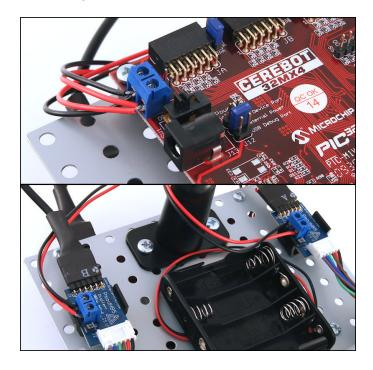
12. Attach the power cable from the battery pack to the J14 battery power connector on the Cerebot MX4cK board.
