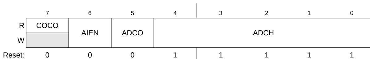
Figure 10-3. Status and Control Register (ADCSC1)
