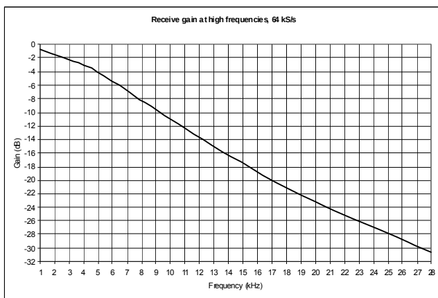
Figure 5. Receive Gain at High Frequencies (600 W)
