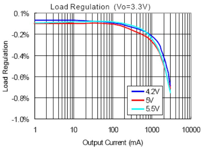
**Typical Performance Characteristics** (cont.) (@ $T_A = +25^\circ\text{C}$ ,  $C_{IN} = 33\mu\text{F}$ ,  $C_O = 22\mu\text{F}$ , unless otherwise specified.)
