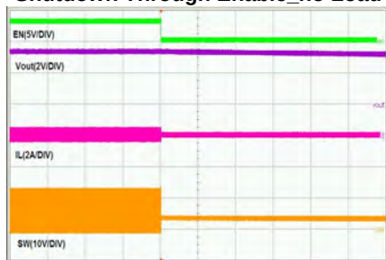
Shutdown Through Enable_no Load
