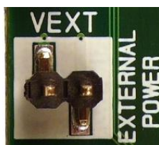
Figure 11 – TrxEB rev. 1.7.0 external power supply header (P1)
