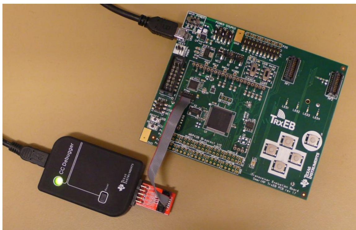
Figure 33 – Proper connection for board resurrection.
