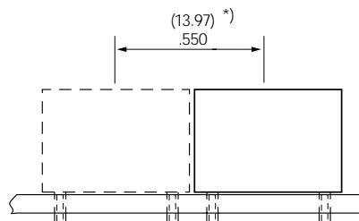
\*) min. pitch between SFF transceiver according to MSA.
