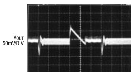
Transient Response (Burst Mode Operation)
