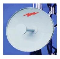
1.2 m | 4 ft Standard Parabolic Unshielded Antenna, single-polarized, unpressurized, 5.725–6.425 GHz, N Female, gray antenna, molded gray radome with flash, standard pack—one-piece reflector
