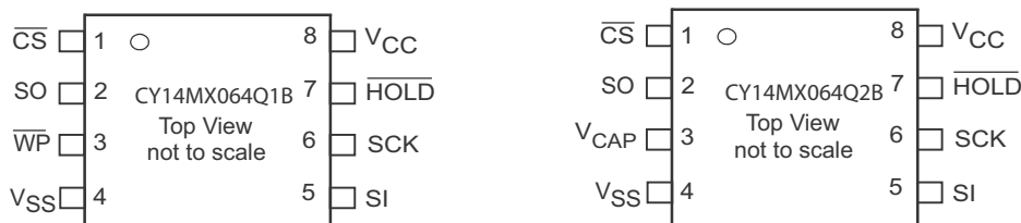
Figure 1. 8-pin SOIC pinout [1, 2]
