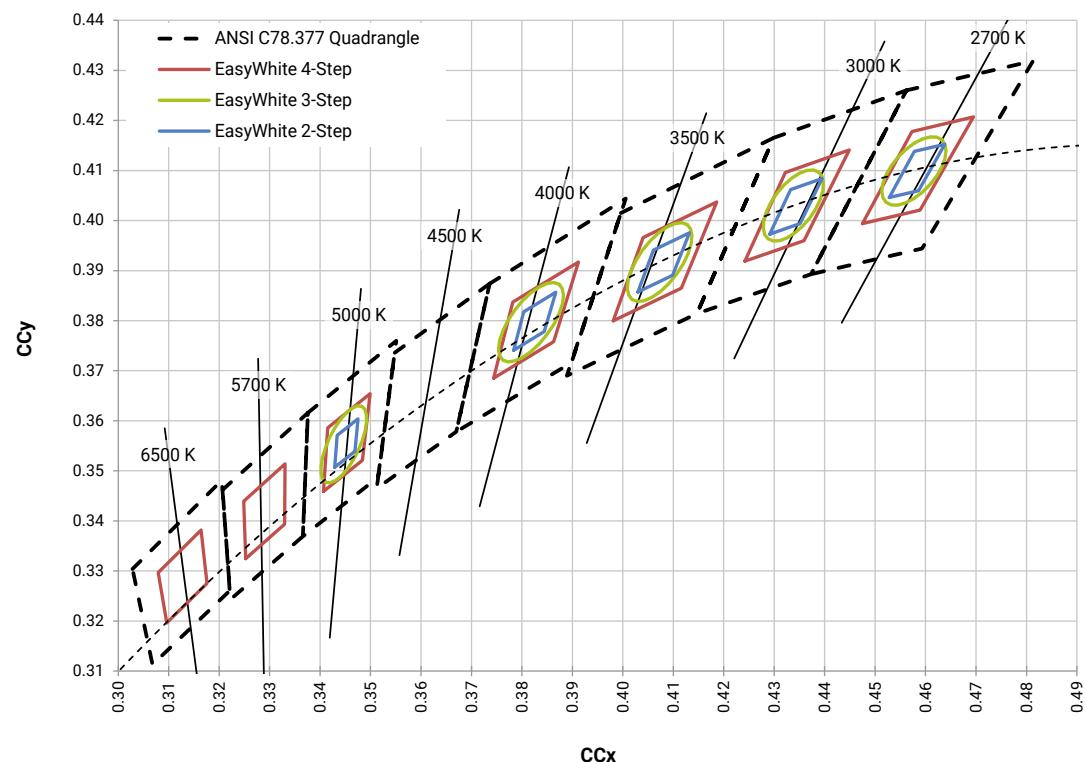
CREE ANSI WHITE BINS PLOTTED ON THE 1931 CIE COLOR SPACE ( $T_J = 85^\circ\text{C}$ )
