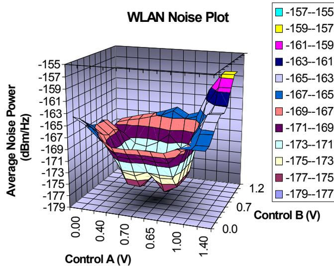
FIGURE 28. 3D NOISE FLOOR PLOT FOR GAIN AND PHASE FAMILY OF CURVES @ 2.4GHz
