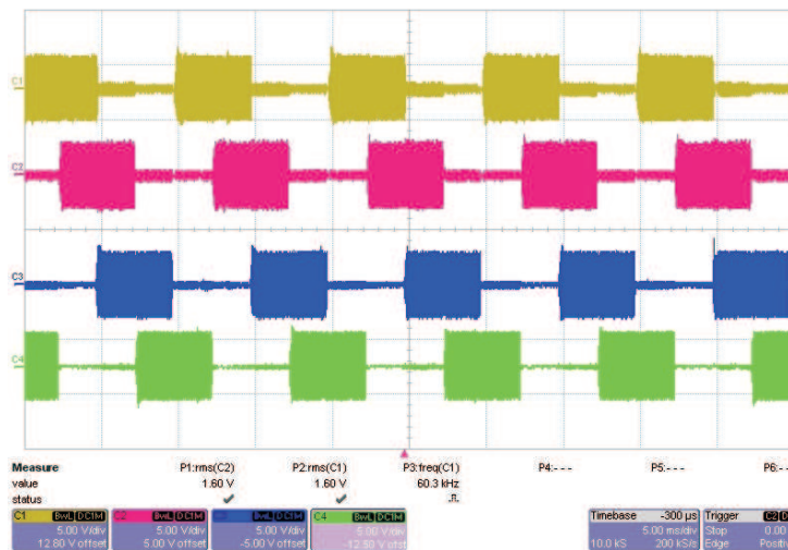
Figure 6. External Burst Dimming, CSEN Test Point Lamps 1, 2, 3, and 4
