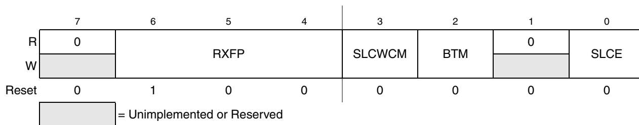
Figure 12-5. SLIC Control Register 2 (SLCC2)
