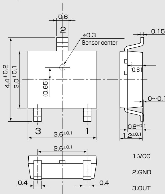
※The sensor senter is located within the  $\phi 0.3\text{mm}$  circle.
