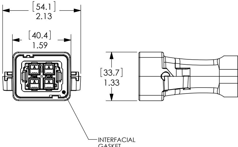
PLUG MATED WITH RECEPTACLE, WITH LATCH MOUNTED ON PLUG
