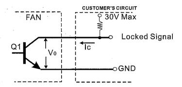
\*Transistor Q1 at "ON" position
