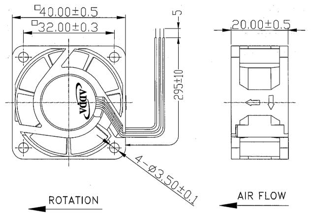
LEAD WIRES: UL 1007, AWG26, L = 295 +/- 10 MM
