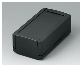
B1060369 TOPTEC 154 H, Vers. I ABS (UL 94 HB) black RAL 9005 6.06"x3.31"x2.20" IP 40
