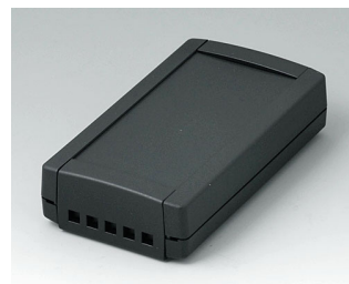
B1055469 TOPTEC 123 F, Vers. II ABS (UL 94 HB) black RAL 9005 4.84"x2.68"x1.18" IP 40
