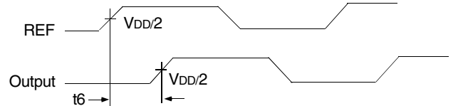
Input to Output Propagation Delay
