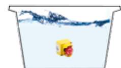
IP67: Submersion to one meter for 30 minutes.
