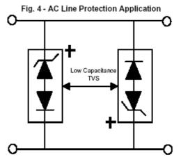
**Application Note:** Device must be used with two units in parallel,opposite in polarity as shown in circuit for AC signal line protection.
