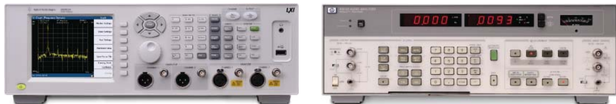
Figure 1. The new U8903A audio analyzer (left) offers numerous improvements over the widely used HP 8903B (right).
