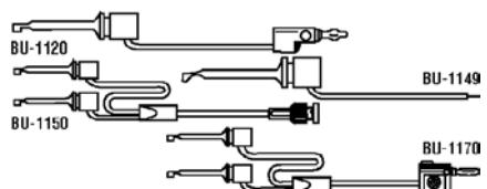
Type BU-1120 attaches to delicate component leads and terminals. Stackable banana plug terminates the other end of test lead. Type BU-1149 to tinned end wire. Type BU-1150 positive and negative with 3' and 8' leads with molded "Y" block to BNC male. Type BU-1170 positive and negative with 3' and 8' leads with molded "Y" block to stackable double banana plug.
