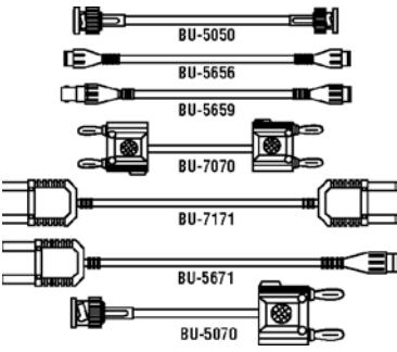
Type BU-5050 has BNC Male Connectors at both ends. Type BU-5656 is the same except features fully insulated BNC Male Connectors. Type BU-5659 is a BNC Male-Female coaxial cable. Type BU-5070 is a BNC to Banana cable assembly. Type BU-7070 has dual banana plugs 0.75" OC on coax. Type BU-7171 features shielded dual banana (0.75" OC). Type BU-5671 combines the insulated versions of both the BNC Male and double banana into the same assembly. All on RG-58 (50 Ω) cable.
