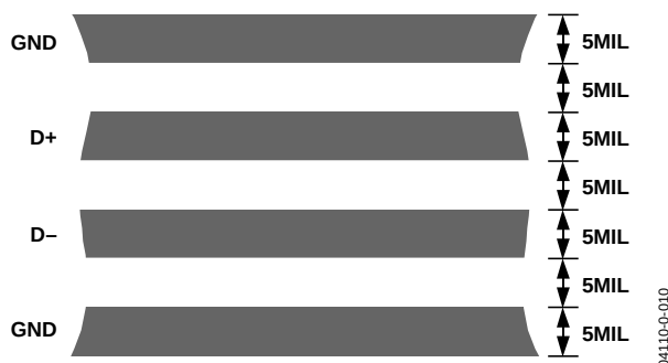
Figure 24. Typical Arrangement of Signal Tracks
